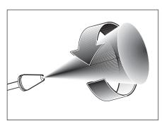
performance of a 0° pencil jet with the surface coverage of a wide angle nozzle. Not recommended for soft materials, siding, painted surfaces, decks or autos.
